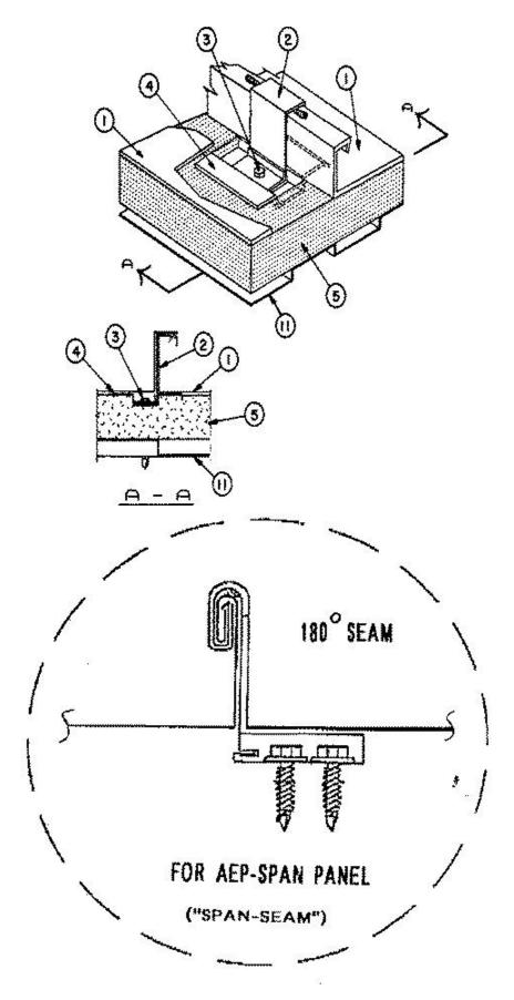
1. **Metal Roof Deck Panels** — \* — No. 24 MSG min gauge coated steel, 16 in. max width. Panels continuous over two or more spans. End lap to occur over purlins and to include End Lap Back-Up Plate (Item 2A or 2B ). Ends of panels
